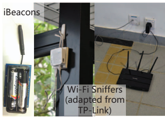
Fig. 8: Illustration of the beacon and Wi-Fi sniffer device settings.
